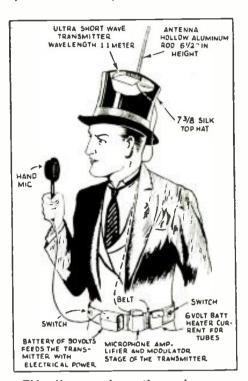
This diagram shows the various component parts of the 1-meter transmitter, the batteries for operating it being carried on a belt around the waist.
