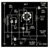
Rf. amplifier using a metal tube.
