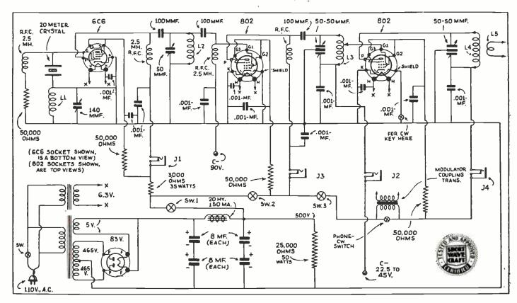
Wiring diagram of the crystal-controlled 5 and 10-meter transmitter, which starts out with a 20-meter crystal. Three screengrid stages are used and modulation is applied to the plate and screen of the "final" amplifier.
