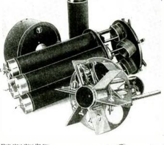
• FOR the past year, concentric cables and parallel transmission lines have been used in transmitters. However, it remained for Frances W. Dunmore of the National Bureau of Standards, Radio Laboratory, to apply these successfully to a receiver.
