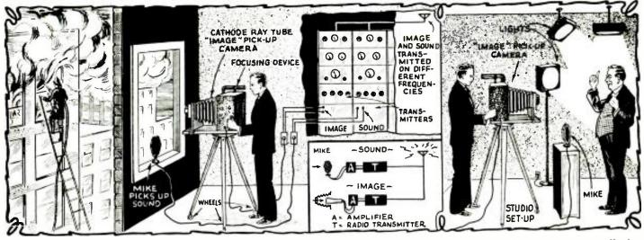
Technique employed in televising outdoor scene. The cut-out in the wall shows the control room and transmitters actually located in an adjacent room. Arrangement of lights, camera, and subject when televising a person in the studio is shown.
