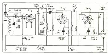
Diagram of 3-tube set using 57, 56, and 2A5.
