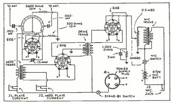
Hook-up of 5 Meter Transmitter (No. 546)
