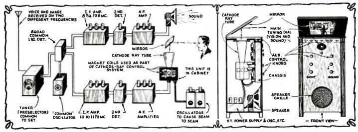
Block diagram of the sight and sound ultra short wave receiver employed in latest television demonstration. Note the common first detector-oscillator system and separate I.F. amplifiers for sight and sound. Sketch of console for sight and sound receiver appears at the right.
