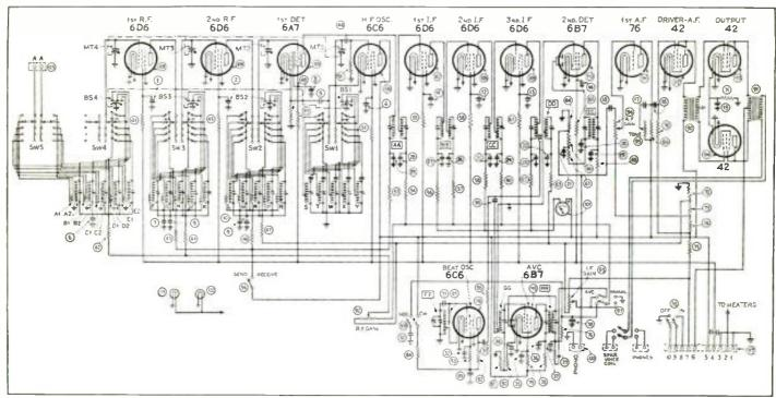
Wiring diagram of the 14-tube "Super Pro" receiver, which possesses the salient features demanded by the expert short-wave "Ham" operator or the critical S-W Listener.
