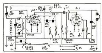
6F7 and 37 used as detector and two A.F.
