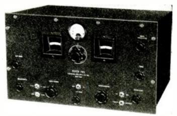
Front view of the Hammarlund "Super Pro" receiver which has a range of 20 mc. to 540 ke. (15 to 555 meters.)
