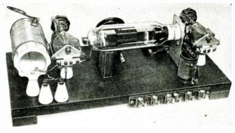
Another view of the oscillator, clearly showing the double-wound filament coil.
