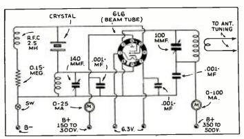
Hookup of Oscillator which makes "quadrupling" possible.
