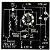
Pentode amplifier using metal tube.
