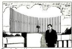
Fig. 6—Portable beam antenna of parabolic shape used by HB9RDL. The chord of the parabola is 3 meters.
