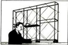
Fig. 8—Curtain antenna for 400 mc. Each section of the radiating and reflecting units of the antenna network is tuned to ½ the carrier wave length. The outer sections of the network are reflectors, while the inner (cubes) are the radiating units.
