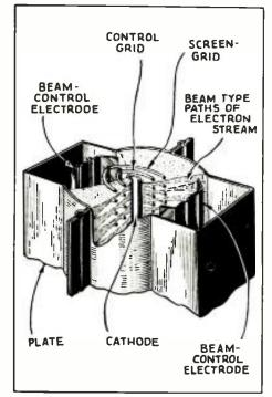
tures of this design are very high-power handling ability and high efficiency, together with high-power sensitivity, permitting a large amount of power output with no grid current flowing in the
