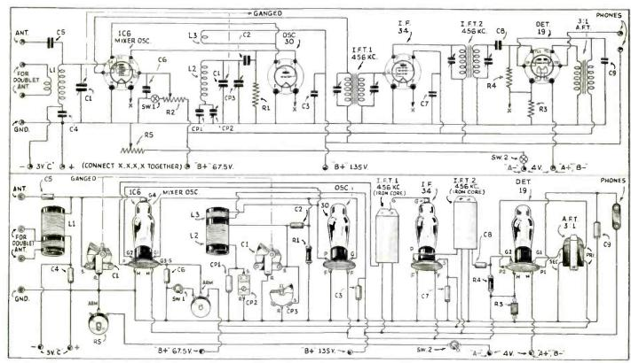
Wiring diagram of the 2-volt short-wave "super-het" receiver. It uses iron-core LF, transformers. Bandspread is obtained, when desired, by using one of the new double-needle "bandspread" dials, such as the Crowe type.
