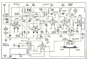
Wiring diagram of the RX-14 receivers
