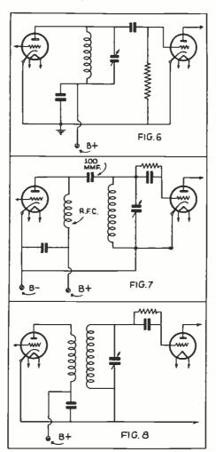
Various types of coupling between two stages of a receiver are illustrated above.
