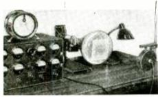
Newest apparatus set-up for testing the luminosity, degree of vacuum, cathode luminosity, degree of vacuum, cathode beam intensity, etc., of cathode-ray tubes.
