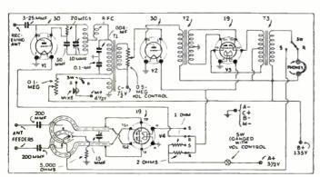
Hook-up of the new 5-meter transmitter-receiver
