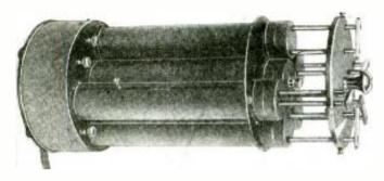
Photo above shows the new ultra short-wave tuning device which employs stiding brass tubes, instead of the familiar coper wire coils, Right—Close-up view one of the concentric tresonant line.
