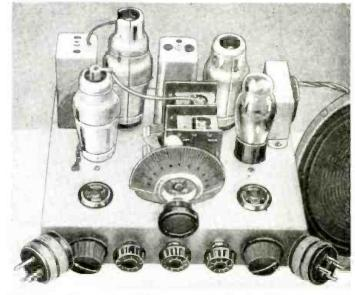
Close-up view of the 4-tube super-het chassis, with two of the plug-in coils.
