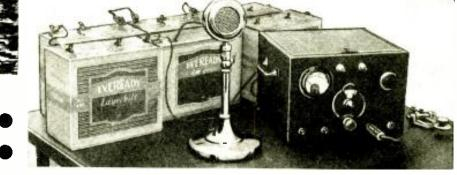
56 mc. Transmitter, with microphone and hatteries, of the type to be used by "Ham" stations in reporting the yacht races on Long Island Sound.
