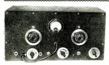
Front View of 5 Meter Transmitter and Receiver
