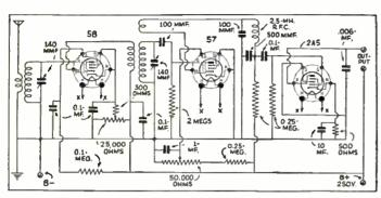
3-Tube receiver using 58, 57, and 2A5.
