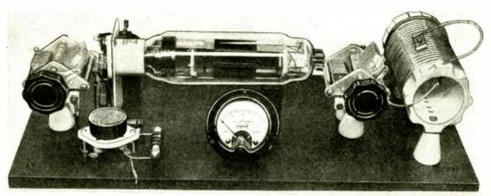
This photograph clearly shows the general layout of the 804 power oscillator.
