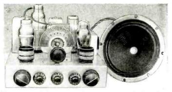
Front view of 2-volt super-het receiver with loudspeaker
