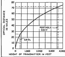
Fig. 1—Theoretical maximum range, on an optical basis, for various heights of the transmitten
