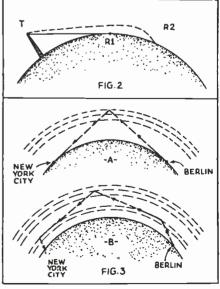
Fig. 2—Illustrating range (R1) of a transmitter T on the assumption of a straight optical path. R2 shows the increase of range of waves following a "bent" path. Fig. 3—Illustrating the effect of reflection from a single ionized layer, and of a combination of refraction and reflection by two separate layers.
