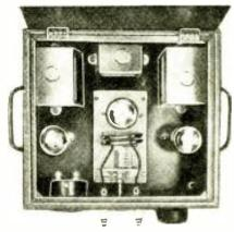
Photos above show close-up and chassis views of the 56 mc. transmitter.
