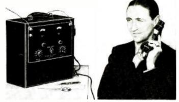
Above—The "Transceptor"—a new 5-meter transmitter-receiver of the portable type shown in use by Mr. Lester. Photos at right show set closed up and below—a rear view, revealing the chassis. No. 544
